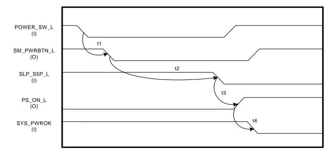
Figure 15. Typical Power-Down Sequence
